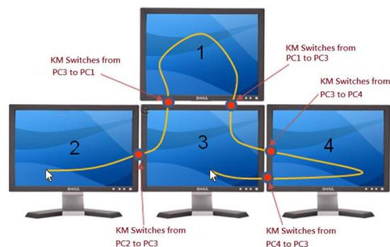
KM Switches are allowing you to seamlessly access up to four computers and their display screens, using a single USB keyboard and USB mouse. The operator can simply move the cursor across screen borders to instantly select the computer they need to control - a great saving in both time and desk space.
